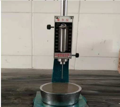
Fig. 3. Experiment on setting time of grouting material
