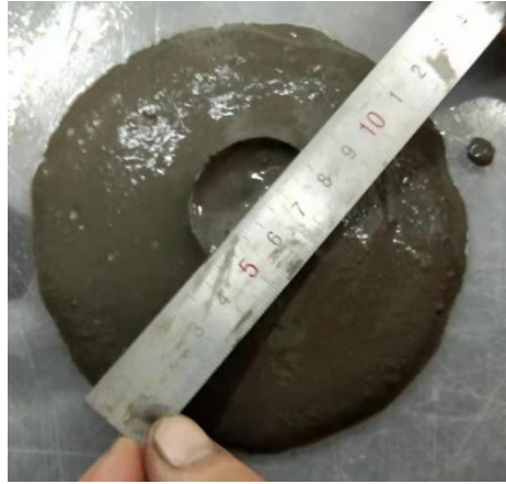
Fig. 1. Liquid flow test of slurry injection
