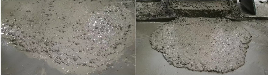
Fig. 2. Fresh concrete before (left) and after (right) adding anti-separation agent
