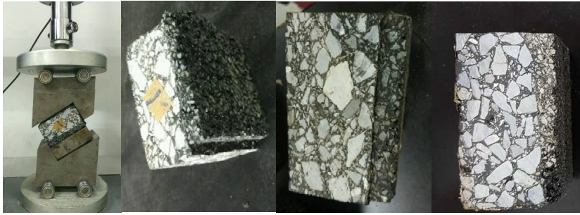
Fig. 6. Diagonal shear tests (from left to right: test method; an LFT UAO specimen after the test; a GT UAO specimen after the test; an RL UAO specimen after the test.)
