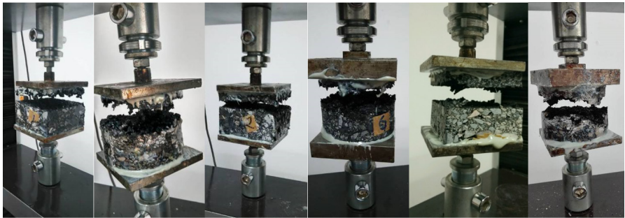
Fig. 4. End tensile tests (from left to right: LFT UAO specimen; LFT core sample; GT UAO specimen; GT core sample; RL UAO specimen; RL core sample.)
