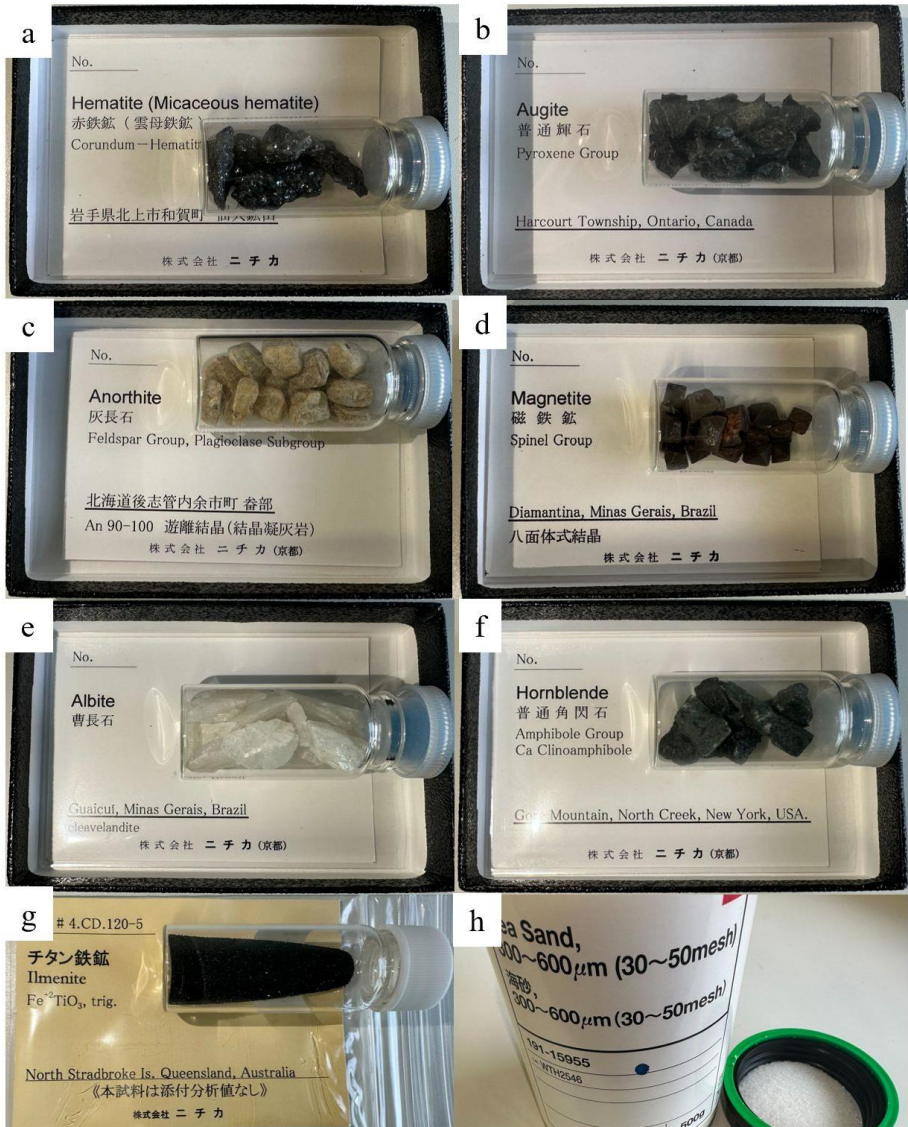
Fig. 6. Rock specimens of Hematite (a), Augite(b), Anorthite(c), Magnetite(d), Albite(e), Hornblende(f), Ilmenite(g), and quartz(h).
