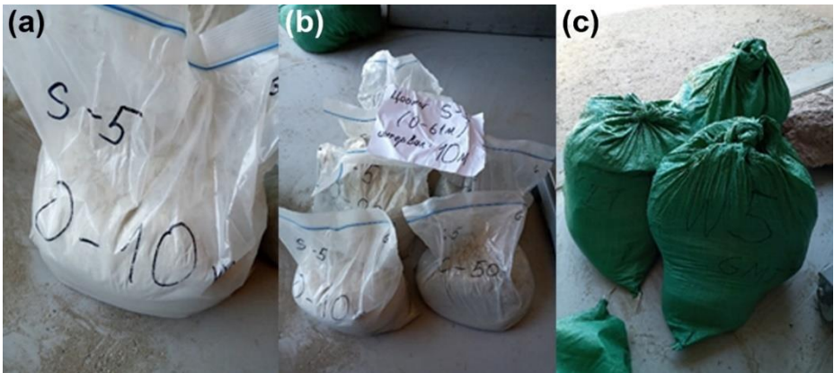
Fig. 2. Drill core samples. (a) an example of the sample identification, (b) an example of the samples packaging with different depths and spots, (c) an example of the spot samples packaging
