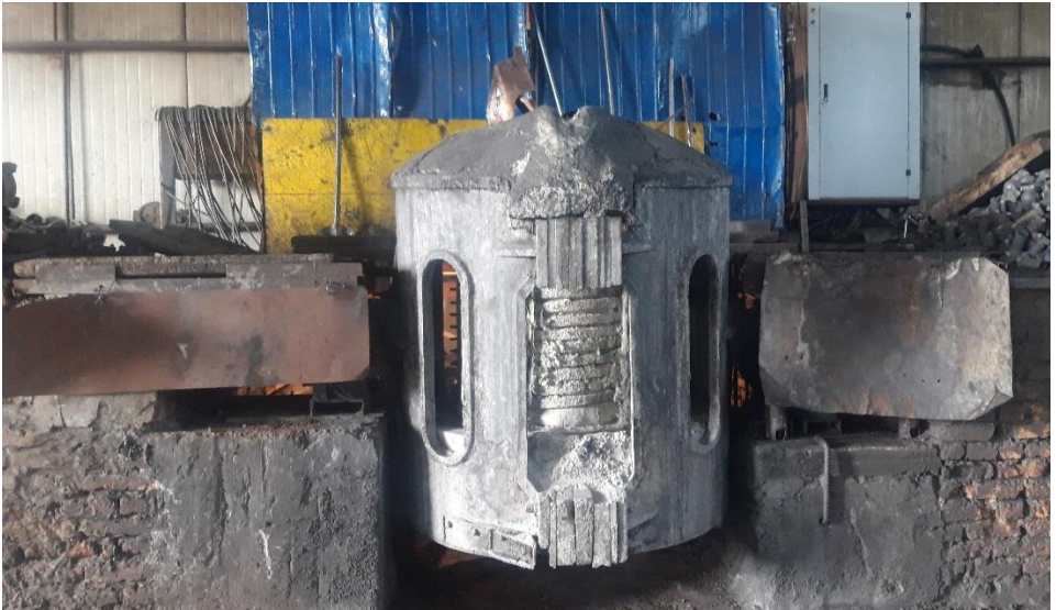
Figure 2. Induction melting furnace at Pelletizing Plant in Nalaikh, Mongolia
