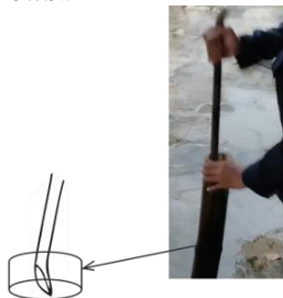
Figure 3. Beveled Surface of the Crowbar
