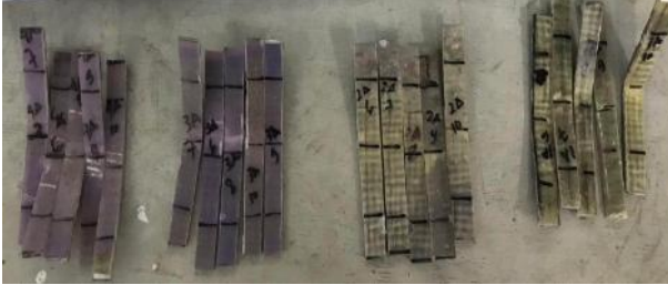
Fig. 2. Specimen prepared for bending test.
