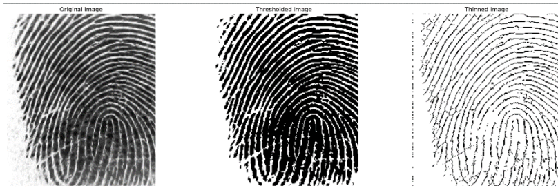
Fig. 3. Thresholding and Thining Process
