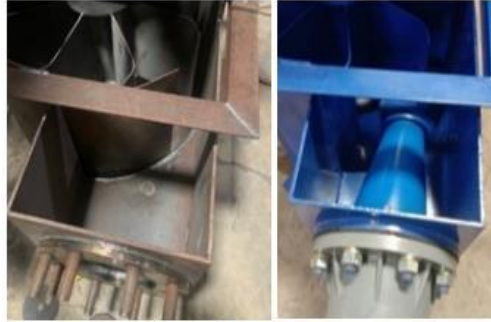
Fig. 5. Turbine Intake (a) Guide Plate (b) Nozzle
