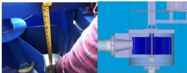
Fig. 7. Runner Position in Turbine House
