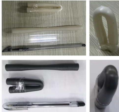
Fig. 10. LDPE (top) and LDPE + 70 % scrap (bottom) specimens before and after bending 180^\circ without initial indication of cracking
