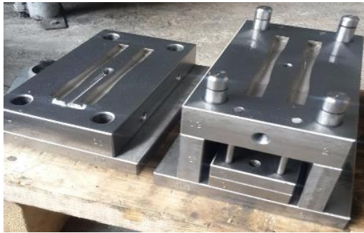
Fig. 2. A set of molds for manufacturing fatigue specimens from PP, LDPE + 70 % Scrap, ABS, HIPS, and PS materials [25]
