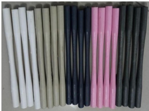
Fig. 3. Injection molding results for 5 types of polymeric materials, PP, LDPE + 70 % Scrap, ABS, HIPS, and PS
