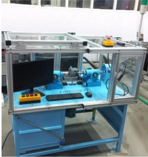
Fig. 4. The integrated rotating bending fatigue testing machine (IRBFTM)
