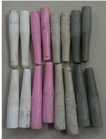
Fig. 5. Some examples of fatigue test specimens after breaking
