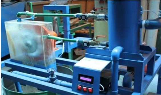
Figure 2 Pelton Turbine Trainer Unit.
