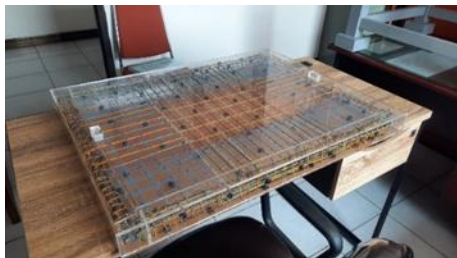
Figure 1 Floor Slab Reinforcement Mockup on the 1:5 Scale.
