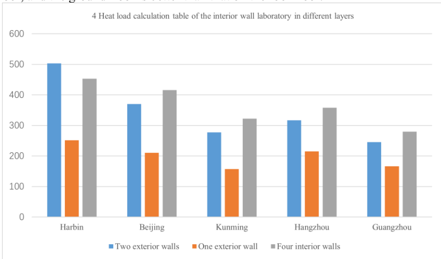
Fig. 4. Four interior walls layout of heat load in different layers in laboratory.
