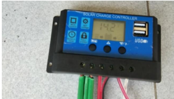
Fig. 3. Solar Charge Controller (SCC)
