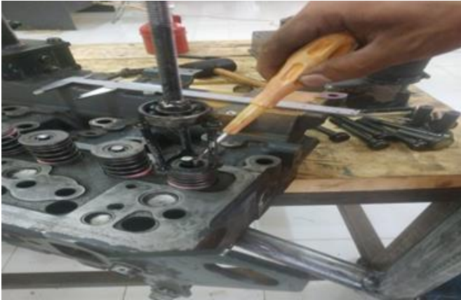
Fig. 5. Spring Valve Opening
