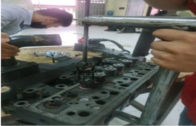
Fig. 7. Spring Valve Installation
