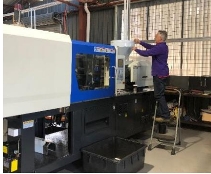
Fig. 1. Manual feed plastic into hopper injection molding by operator [1]
