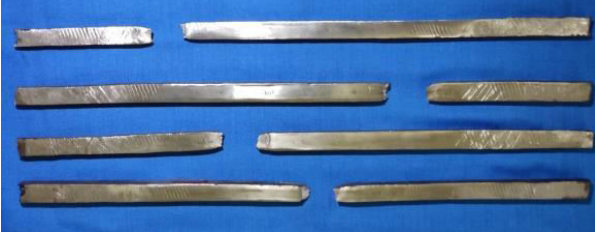
(b) Specimen SP-1/2/3/4 (100A/14.6V) with heat input of 1.86 kJ/mm
