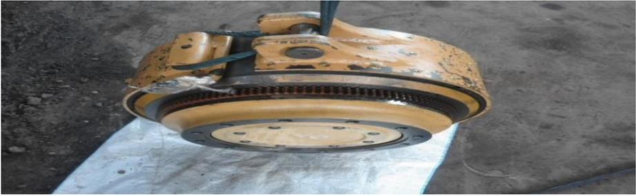
**Fig. 4.** Clutch Assembly Disassemble.
