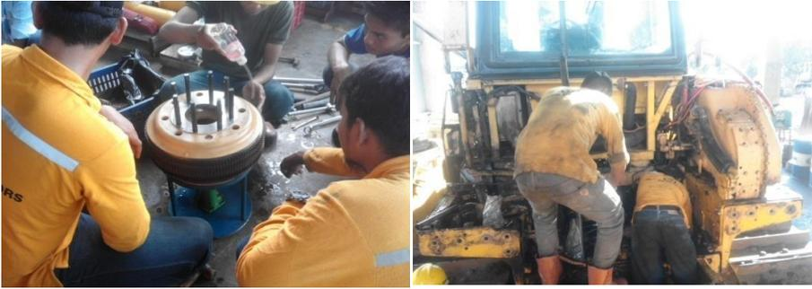
**Fig. 6.** Steering Clutch Repair and Installation Process
