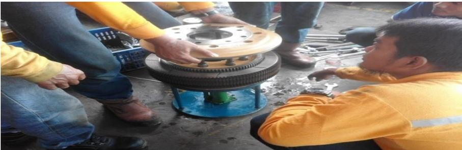
**Fig. 3.** Steering Clutch Assembly Removal.
