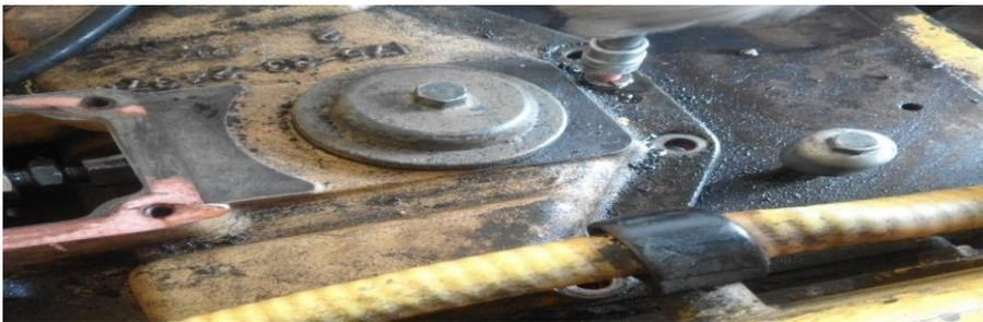
**Fig. 1.** Adjustment Bolt Rod Brake.
