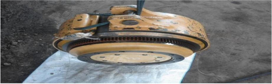
**Fig. 4.** Clutch Assembly Disassemble.
