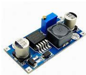
Fig. 7. LM2596 DC-DC Adjustable step down[7]
