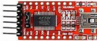
Fig. 2. USB to TTL Module[3]
