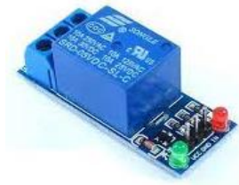
Fig. 3. Relay 5V Module[4]
