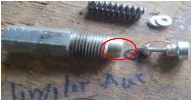
Fig. 3. Pressure limiter valve guide
