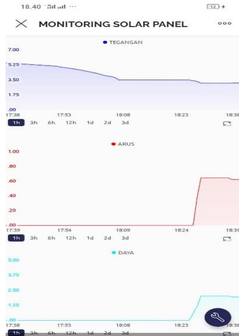
Fig .10. Solar panel monitoring curve with load
