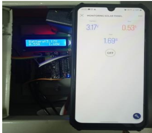
Fig. 8. Display of voltage, current and power monitoring tools with load
