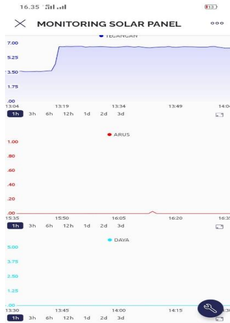
Fig. 9. No-load solar panel monitoring curve
