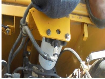
Fig. 3. Fuel filter installed on the troubled unit
