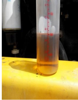
Fig. 6. Injector fuel return measurement
