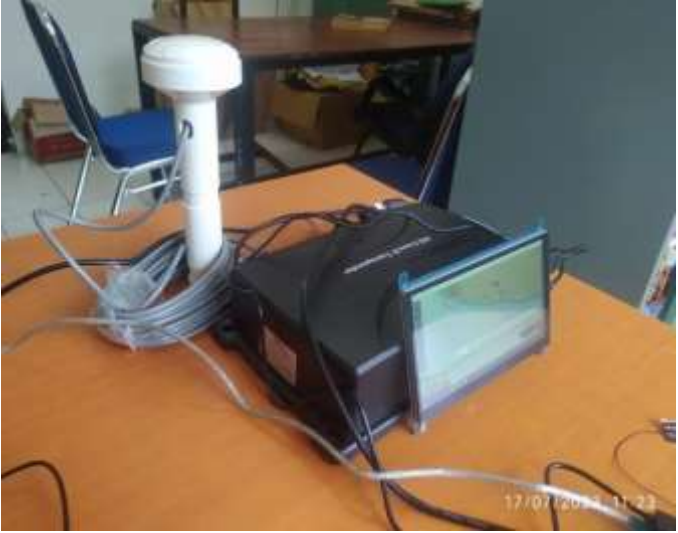
Fig. 4 AIS transponder design result
