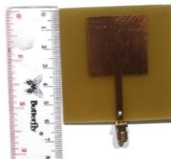
Fig. 4. Realization of 1 element microstrip antenna array with a square patch planar array technique
