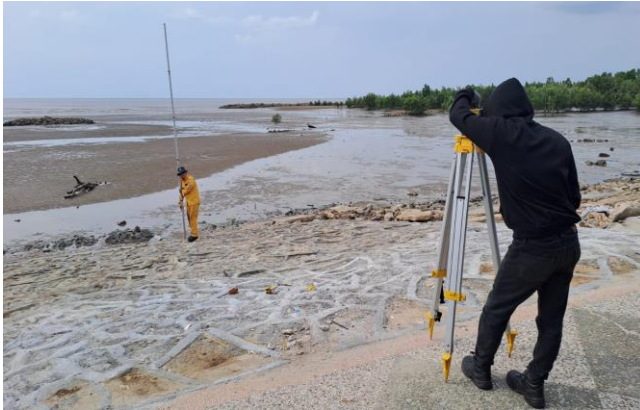
Fig. 6. Seawall slope measurement
