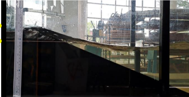
Fig. 15. Wave testing on seawall slope 1:3
