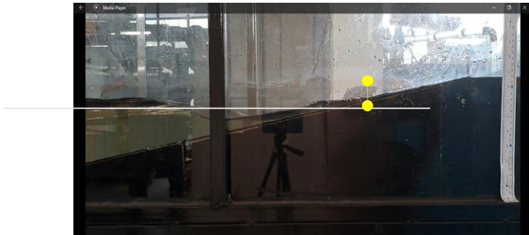
Fig. 16. Wave testing on seawall slope 1:5
