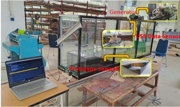
Fig. 11. Seawall structure testing in the Laboratory
