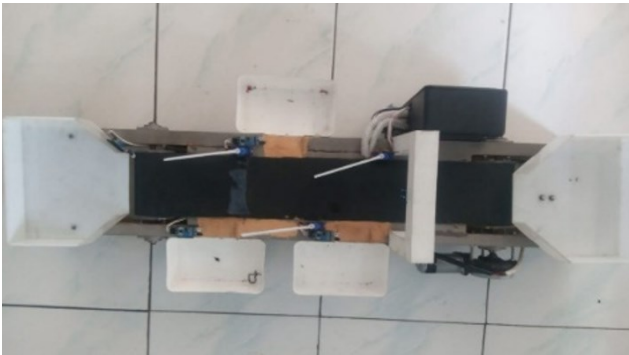
Fig. 5. Top View Conveyor System
