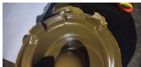
Fig. 1. Flash defect in wax
