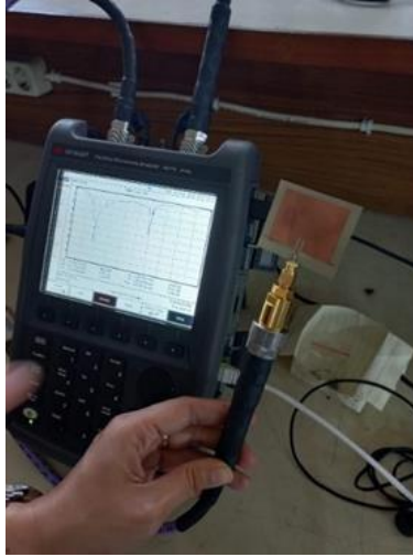
Figure 5. Antenna measurement using a vector network analyzer
