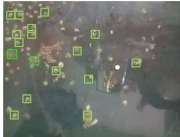
Fig. 14. Detection Biofouling Using Haar Cascade Classifier
