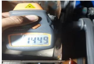
Fig 8. Pully speed measurement
