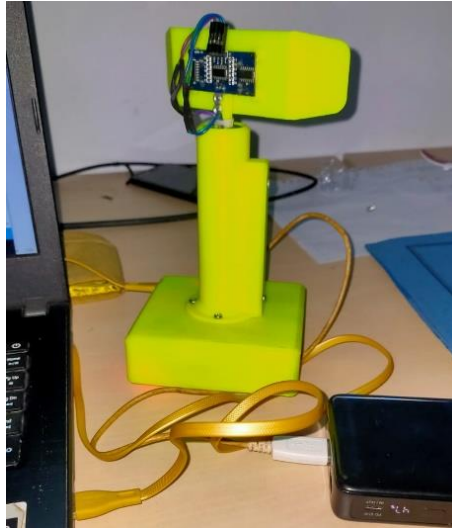
Fig. 4. Step 1: Connect the cable to the laptop and the power supply from the radar
