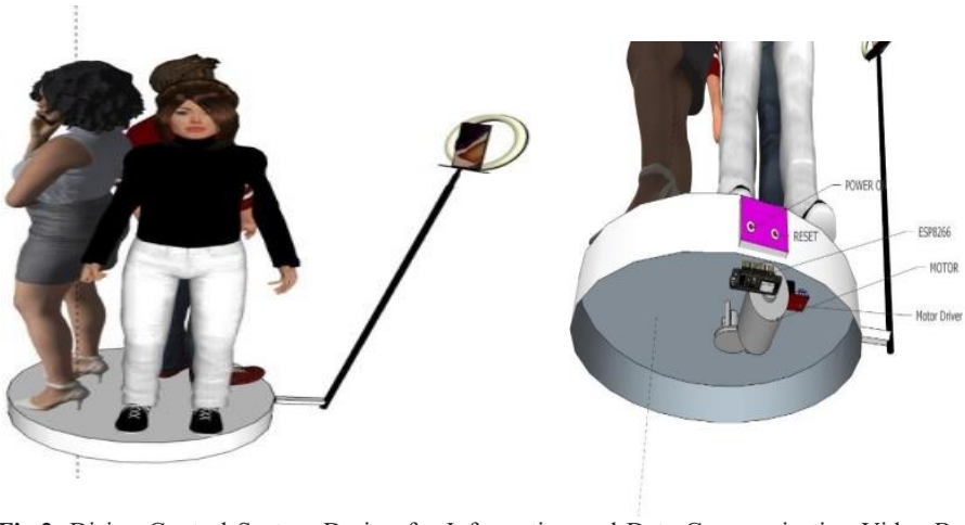
Fig.3. Disign Control System Design for Information and Data Communication Video Booth 360° Using Internet of Things Media
