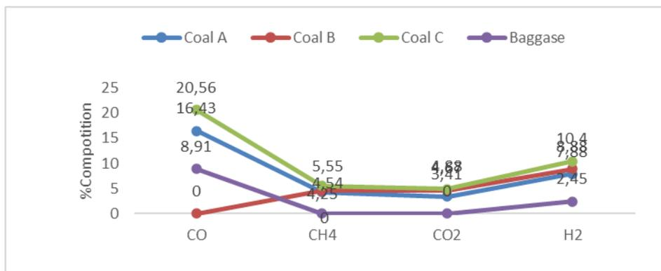
Figure 1. Graph of syngas composition from coal and bagasse
