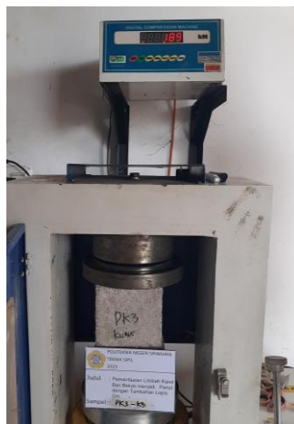
Figure 4. Cube Compressive Strength Testing
