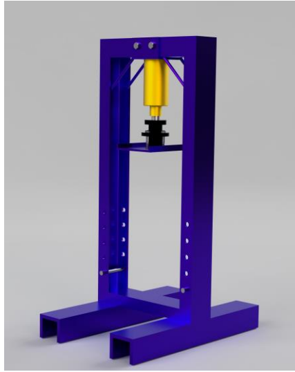
Figure 3. Vertical Load-Bearing Frame
