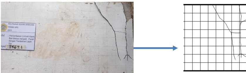
Figure 8. PKGT1 Test Object Damage Pattern
