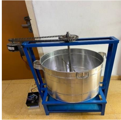
Fig.3. Semi Automatic Batik Fabric Dyeing Equipment Multiplied Natural Fiber Typical In Palembang Based on Internet of Thing
