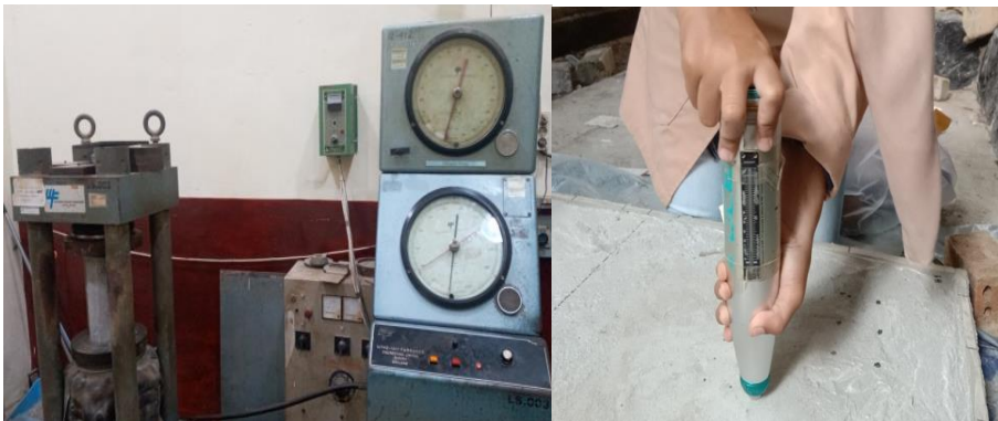
Figure 2. Laboratory Concrete Compressive Strength Testing and Testing of Reinforced Concrete Slabs Using Hammer Test
