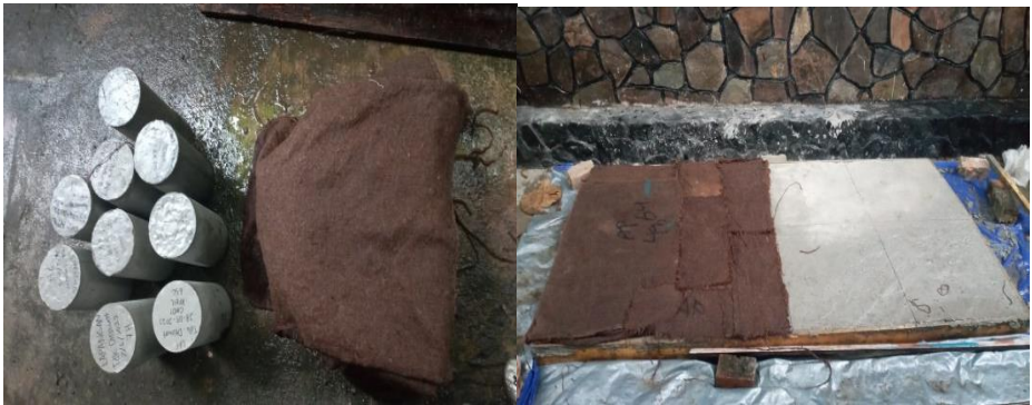
Figure 1. Cylindrical Test Object and Reinforced Concrete Plate Test Object
