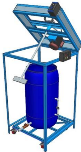
Fig 1. Design Mixer Machine for Liquid Soap Making Machine with Capacity of 160 Liters
