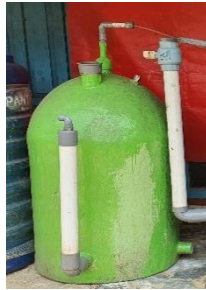
Fig 2. Fixed Dome Biodigester
