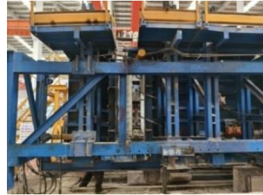
(b) longitudinal installation of end formwork
