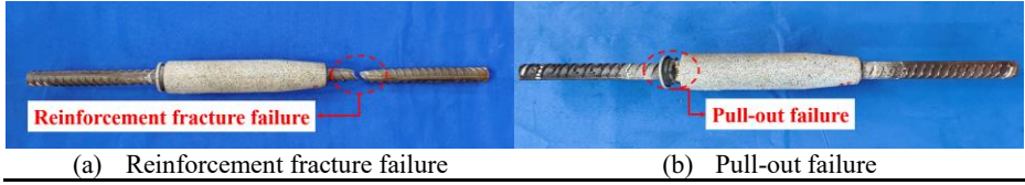
Fig. 6. Comparison of typical failure modes.
