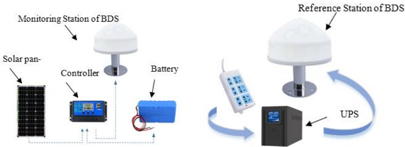
Fig. (a) Monitoring Station of BDS Figure (b) Reference Station of BDS Fig. 2. Composition of BDS Monitoring Station and Reference Station
