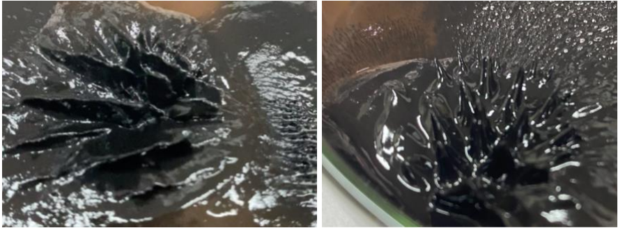
Fig. 1. (a) photocopy toner-based ferrofluid; (b) magnetite-based ferrofluid
