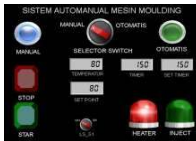
Fig. 19. HMI inject is not activated manually
