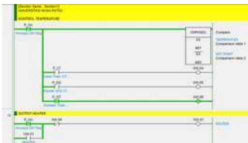
Fig 9. The heater test program is controlled by a thermocouple sensor in OFF condition
