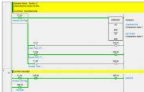
Fig 7. The heater test program is controlled by the thermocouple sensor in ON condition
