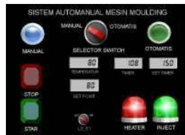
Fig 17. HMI inject activates manually
