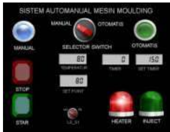
Fig 8. HMI heater and temperature ON
