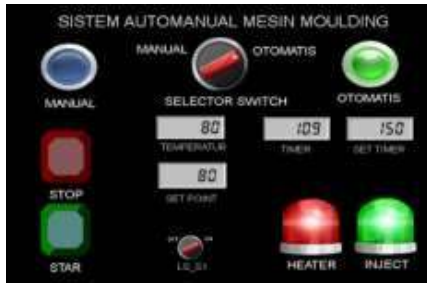
Fig 13. HMI inject is active
