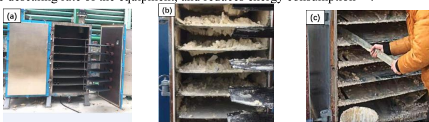
Fig. 3. A typical cabinet manual descaling device (a) Before use; (b) After water softening treatment; (c) Manual descaling
