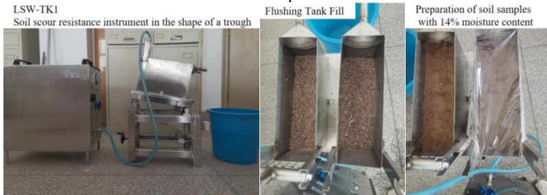
Fig. 1. Schematic diagram of experimental apparatus and filling soil
