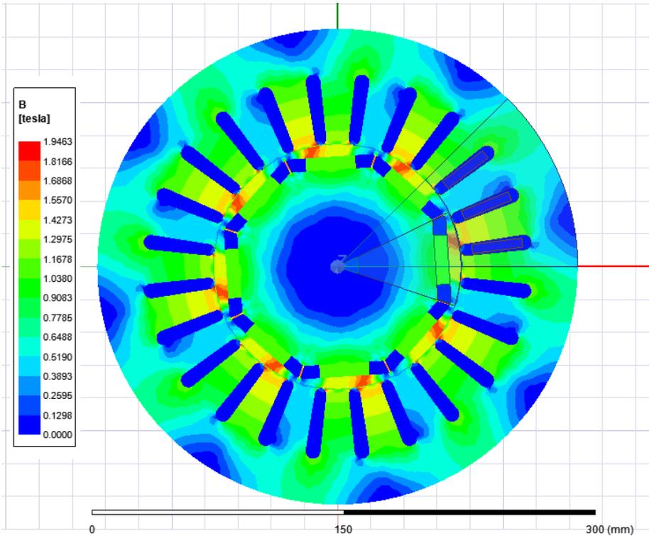
**Fig.2** Flux density in motor - magnitude
