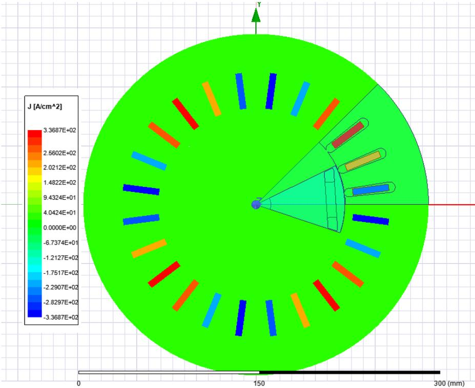
**Fig.4** Current density in motor
