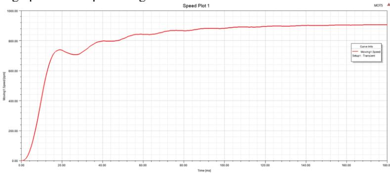
**Fig.5** Motor speed - calander characteristics
