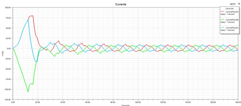
**Fig.7** Currents in stator winding
