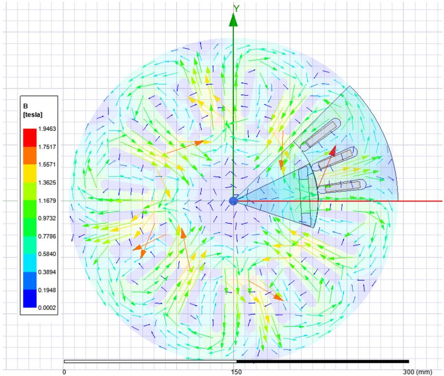
**Fig. 3** Flux density in motor - vector flux
