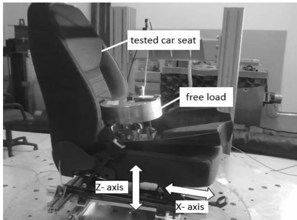
Fig. 1. The principle of a car seat testing.
