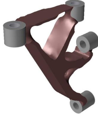
Fig. 8. Results of topology optimization in Altair Inspire with partitions – Altair Inspire 2
