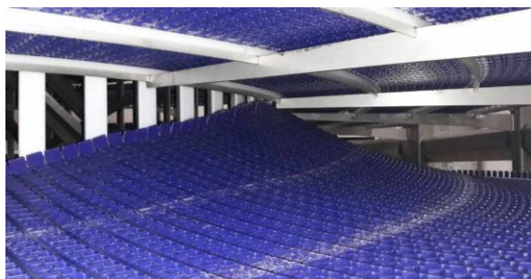
Fig. 6. Lifting the belt on inside radii as a result of higher tension on top of first tower.
