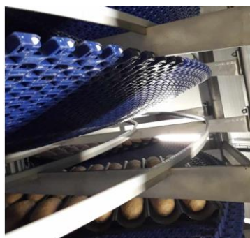
Fig.7. Lifting the belt on outside radii as a result of incorrect speed of drums.
